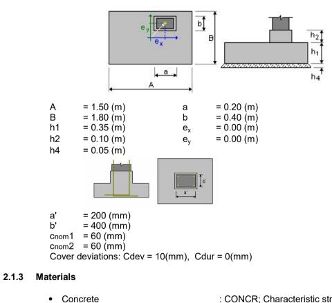
: CONCR; Characteristic strength = 20.00 MPa Unit weight = 2501.36 (kG/m3) Rectangular stress distribution [3.1.7(3)] : type T Characteristic strength = 460.00 MP
